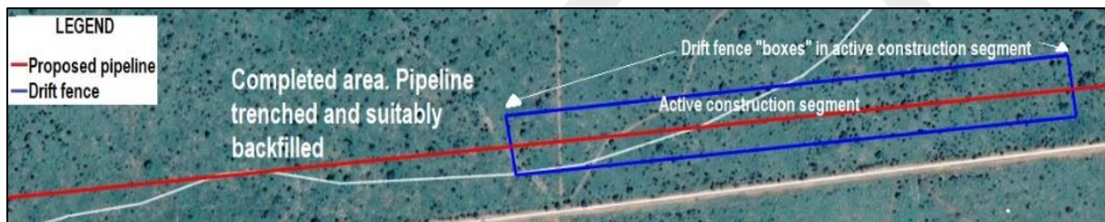
Figure 1: Example off how drift fences must encompass the active construction segment of the pipeline.
