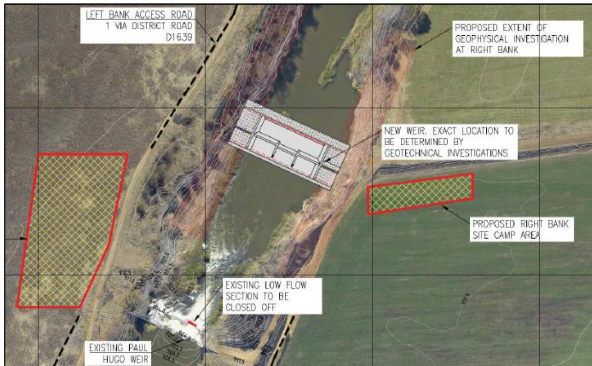
Figure 4: Layout plan of A2H116/132 and concept layout of proposed new weir downstream of Paul Hugo
